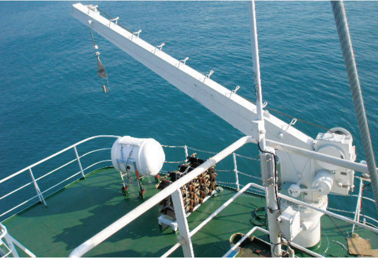
Single arm slewing type - electric/hydraulic
