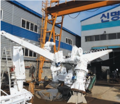
Rescue boat & provision handling davit - electric/hydraulic
