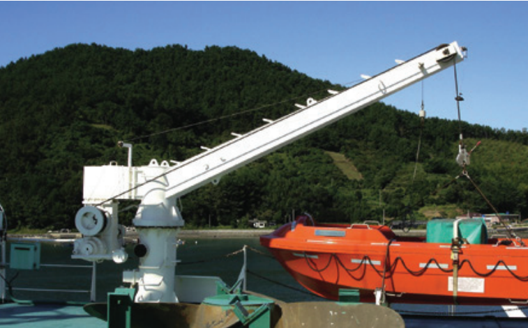
Single arm slewing type - electric/hydraulic
